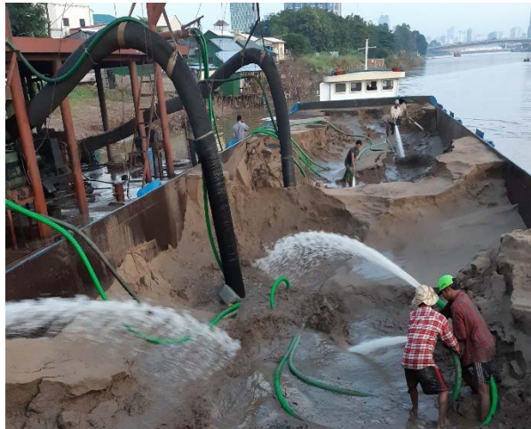
Figure 3. Labourers blast water at sand in order to dislodge it so it can be pumped out of the barge through large tubes. Up to ten labourers work for an hour to empty one boat. They often live and sleep at the pumping station (October 9, 2019)
